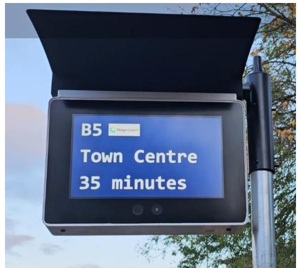
Figure 7 – Image of one of the new RTPI displays
